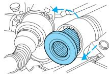
5. Replace the two halves of the air filter housing and secure the clamp.
